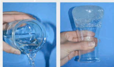
Fig. 4. Left hand side 1% thiolated poly(acrylic acid) solution before oxidation and right hand side after oxidation
